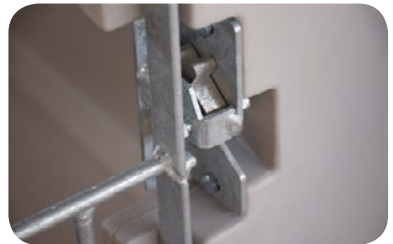
Slam latch locking mechanism that keeps the calf safe.
